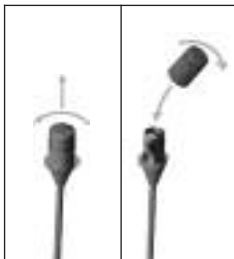
Fig. 10: Mounting the PB 77 presence boost cap.
